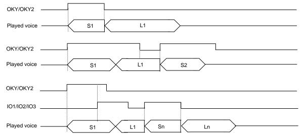
While playing OKY's Looping voice (L1, key is released), triggering OKY or IO1 is active in Retrigger mode.
