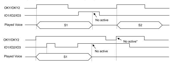
$\divideontimes$  Because IO1 signal is still high, the OKY Edge signal is not active.
