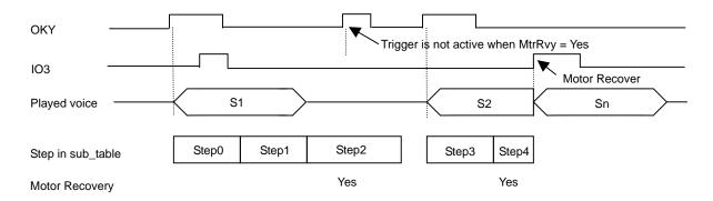
OKY (E/U/R) = S1 S2, (S1 = step0 + step1 + step2 (Jump to Mute), S2 = step 3 + step4), IO3 (E/U/I) = Sn
